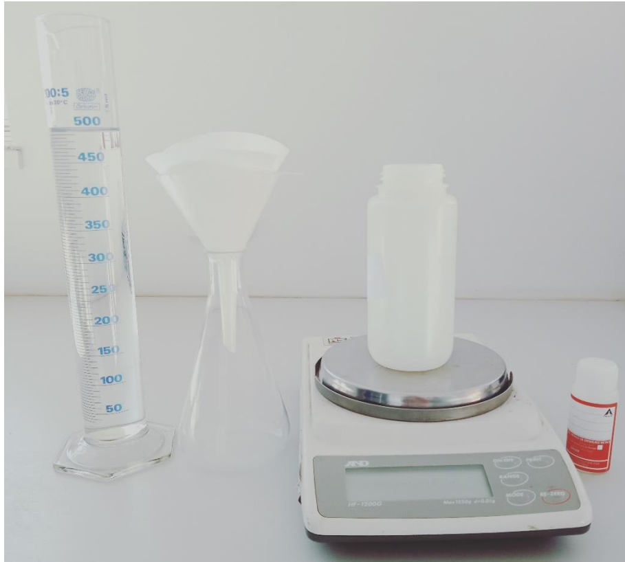
Figure 103: Experimental equipment used in the USGS field leach test method
