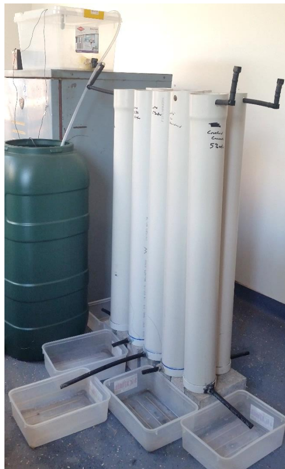
Figure 20: Cluster of biofilter simulation column apparatus depicting single PVC monophasic column arrangement, underdrain tubing and effluent collection trays (Macnamara 2015)
