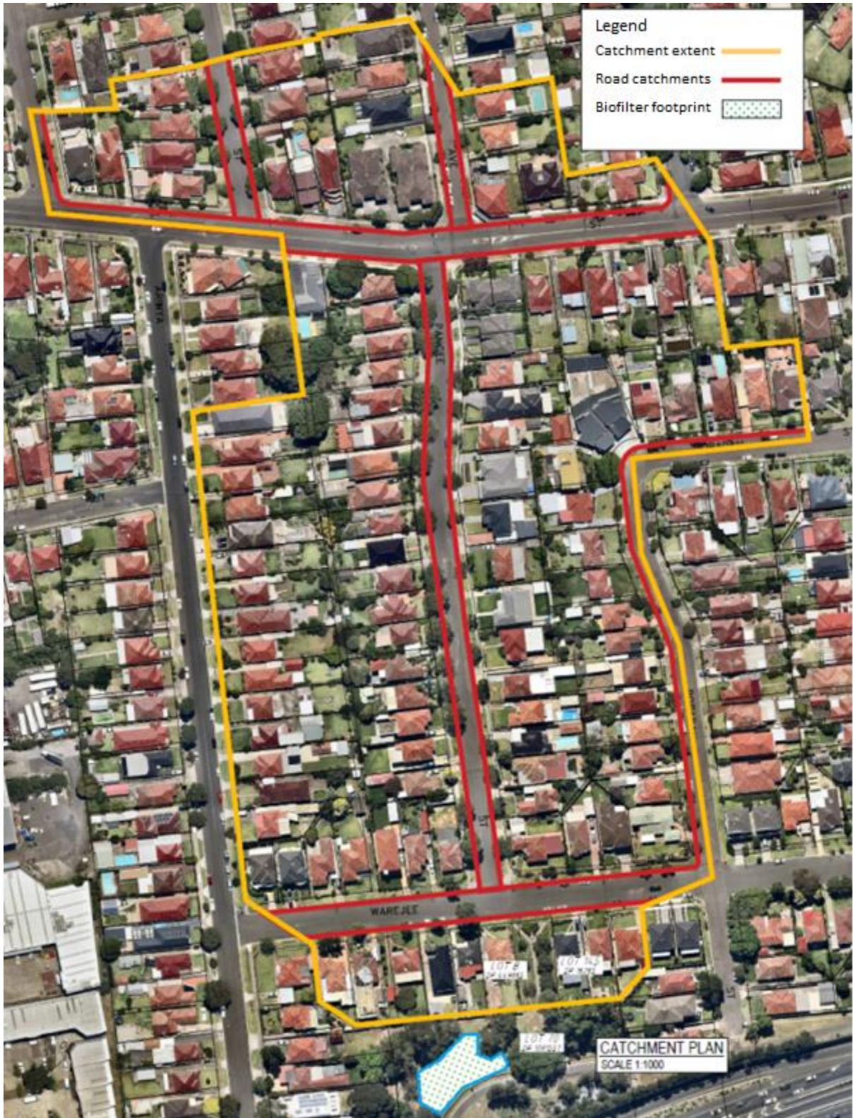
Figure 7: Biofilter at Kingsgrove, NSW and its catchment to illustrate typical size relationship (Cooks River Alliance, 2016)
