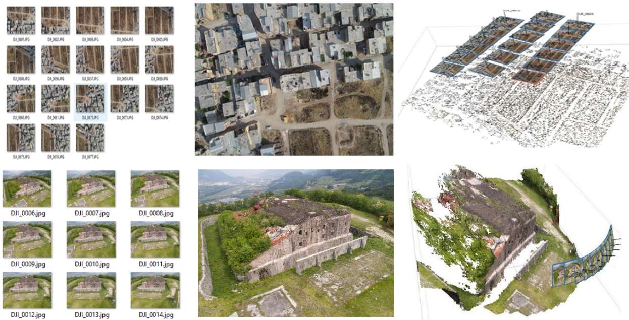
Figure 10. The real datasets used in the evaluation: multiple overlapping strips with 18 images (top) and 9 convergent images (bottom).
