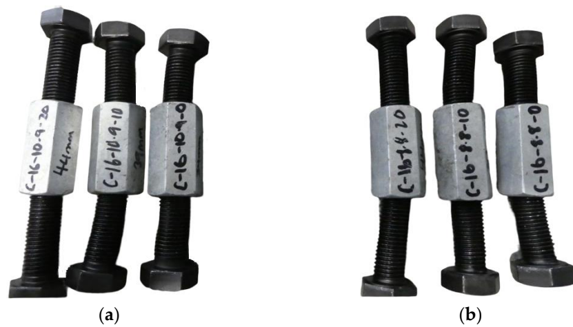
Figure 7. Failure modes of M16 bolts with 8.8 grade coupler. (a) M16-10.9 bolts. (b) M16-8.8 bolts.
