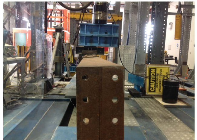
Figure 17: Distortional buckling within flange.
