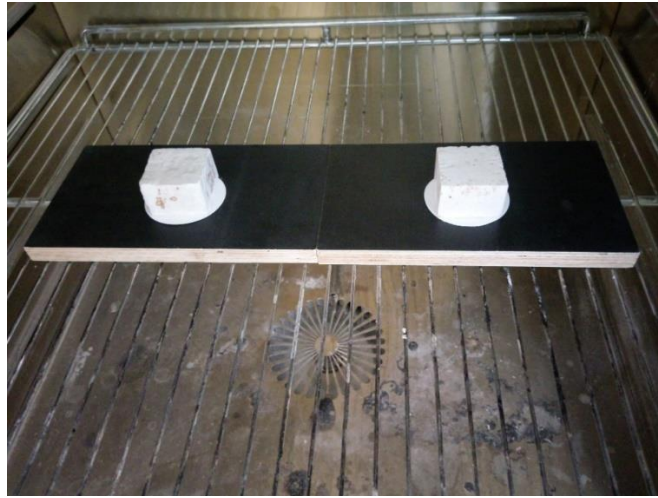
Fig. 4.1. Specimens subjected to leakage testing at 40 and 70 °C.
