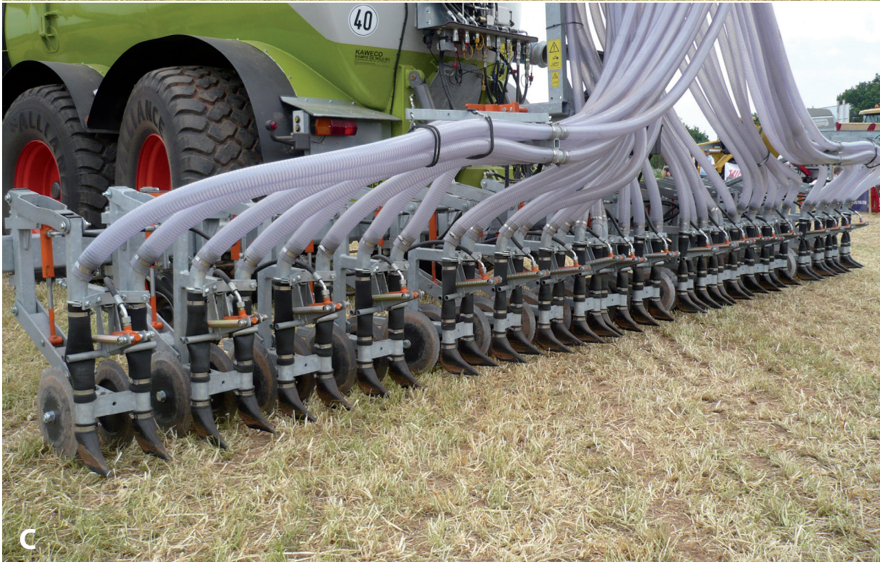
Image 18: Comparison of three types of low-emission spreader for liquid manure or 'slurry' (Field Measures 6 and 7). (A), 'trailing hose' exits just above the ground; (B), 'trailing show' deposits slurry on the soil surface, below the canopy; (C), 'injection system' inserts manure into the soil through a slot cut by the preceding wheel (photograph: © ADAS).
