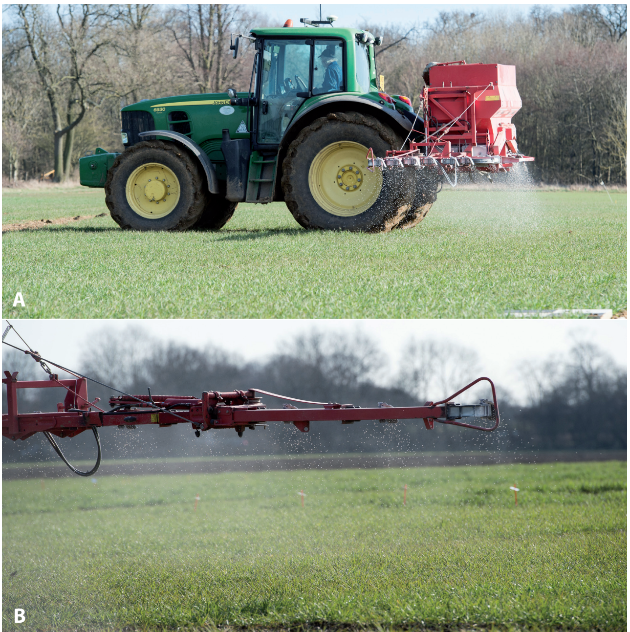
Image 15: Precision fertiliser application (supporting Field Measure 2). In advanced systems, individual sections across the boom width can be turned off (B), so that combination with a global-positioning system (GPS) during the spreading operation can be used to avoid overlap or to calibrate dose according to requirements based on leaf-colour sensing (photographs: © Rothamsted Research).
