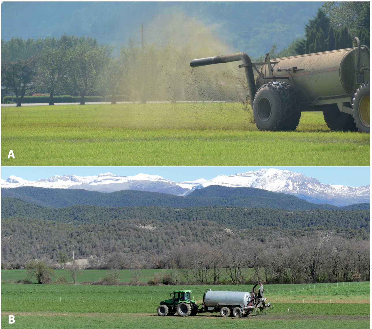
Image 16: Comparison of slurry spreading with a traditional ‘splash plate’ spreader ( A ), maximizing ammonia emissions, (photograph: © Shabtai Bittman) with a trailing hose manure spreader ( B , Field Measure 6) for reducing ammonia emissions, here deployed on-farm in a sensitive mountain landscape. For optimal performance, hose exits should be set within 15 cm of the ground, though they may be raised when turning or transporting manure from the farm (photograph: © L’Albeitar, 2021).
