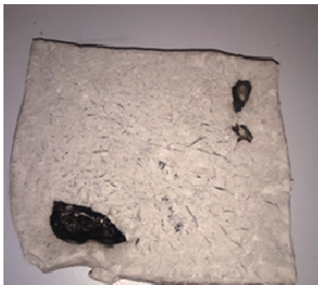
Figure 2 CAA20 sample obtained with non-desirable properties after 15 h of sublimation under vacuum.
