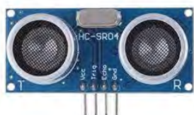
Figure 2. Schematic of an Ultrasonic ranging module HC-SR04 (Kamal and Hemel, 2019)
