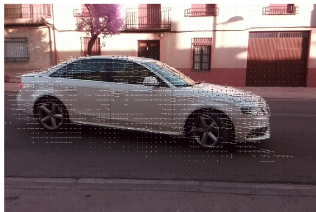
Fig. 2. Example of motion vectors obtained using the developed device.
