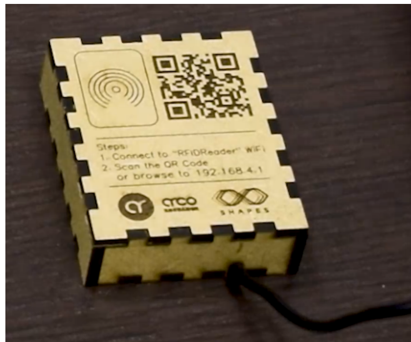
Figure 7. Wristband RFID writer device.
