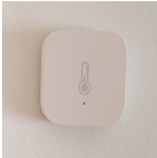
Figure 21. Temperature and humidity sensor to monitor comfort in a room.
