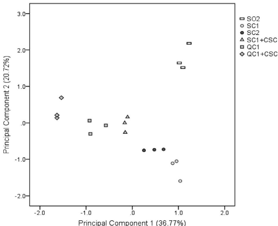
Fig. 1. Plot of wines treated with SO<sub>2</sub> and natural extracts, with or without colloidal silver complex, distributed in the space defining by principal components PC1 and PC2 with regard to significant volatile compounds.
