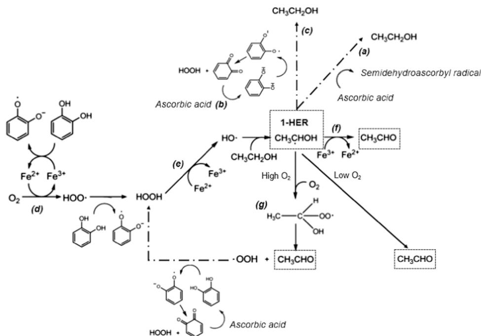
**Figure 5.** Scheme proposed to explain the possible pathways of the ascorbic acid for the inhibition of 1-hydroxyethyl radical and the formation of acetaldehyde. Adapted from Elias and Waterhouse.<sup>13</sup>
