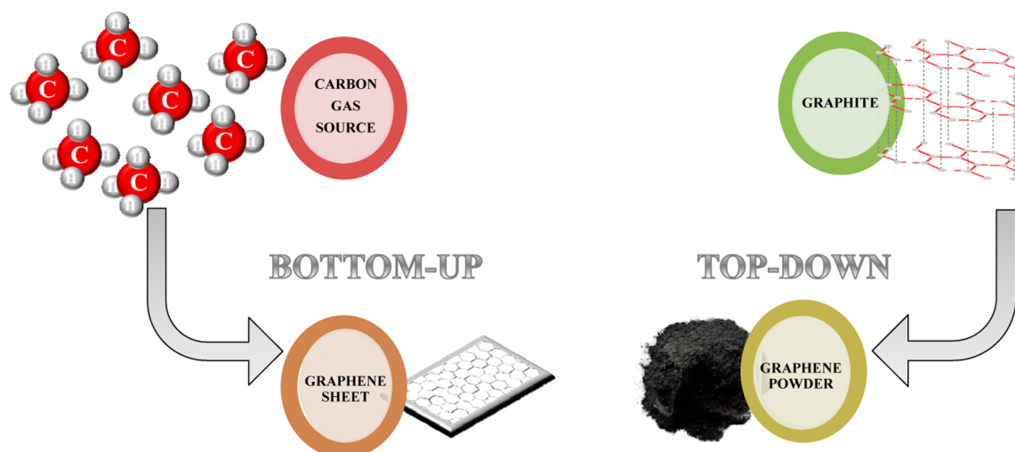
Figure 3. Bottom up and top down routes to synthesize graphene.
