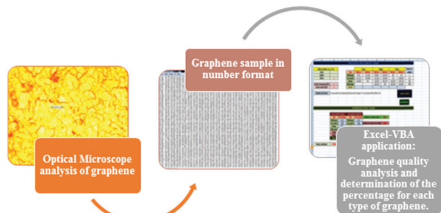
Fig. 2 Excel-VBA application to determine the percentage of each type of graphene and the graphene quality value.
