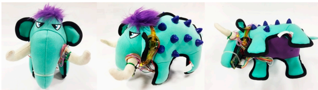
Figure 2. Non-intrusive integration of the hardware with MAMIoTie.
