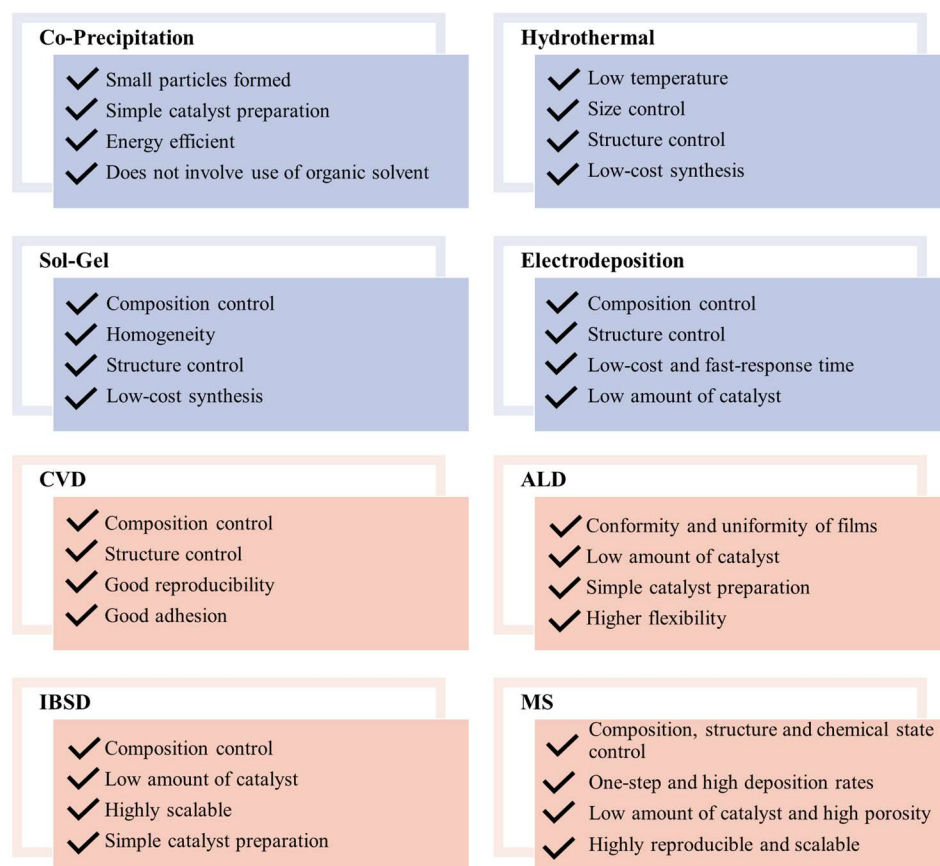
Figure 8. Summary of the main advantages of the catalyst deposition processes regarding their implementation in AEMWE.
