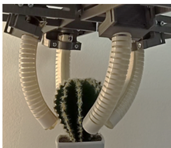
Figure 1: Soft robotic hand with hydrogel-based pneumatic actuators.
