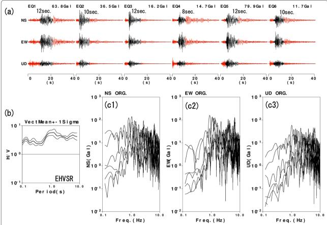
**Fig. 2** Process to evaluate EHVSR at TTR002 site. **a** Three component acceleration waveforms of used records with PGAs and window lengths of analysis. Red color shows the full waves and black shows the windowed waveforms. **b** Average and ±1 standard deviation of EHSVR derived from the panel **c1–c3**. **c1–c3** show three component Fourier spectra of the target records that are used to evaluate EHVSR
