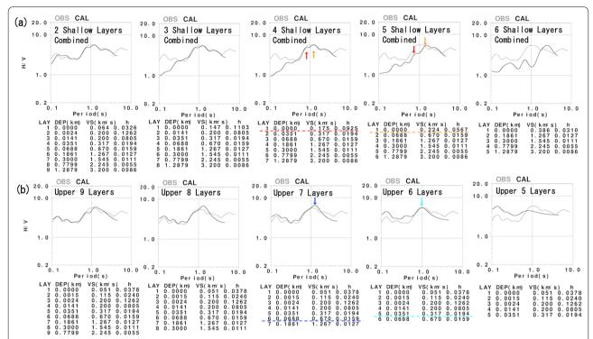
**Fig. 4** a Calculated EHVSR by combining the surface layers in order from the shallow layer with evaluated average S wave velocity of target layers. Red and orange arrows and dashed lines indicate the characteristic periods and the layer boundaries that compose them. **b** Same as upper row but for removing the deepest layer from the previous model. Blue and sky arrows and dashed lines also indicate the characteristic periods and the layer boundaries that compose them
