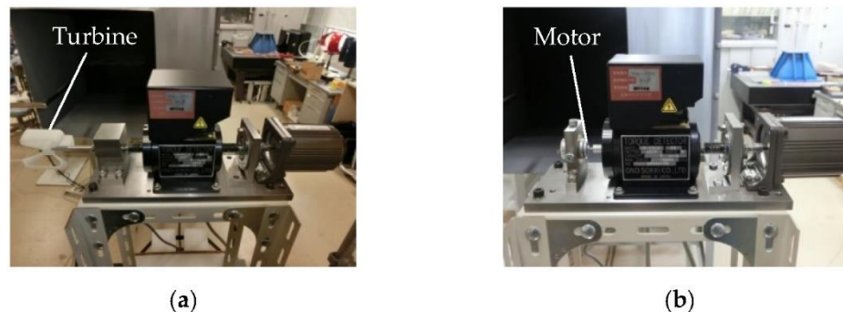
Figure A1. Experimental setup of the torque measurements at Tottori University (viewed from downstream): (a) a miniature wind turbine model; (b) a direct current motor with no current.
