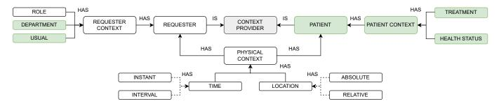
Fig. 2. The context model employed to build risk-based access control policies.
