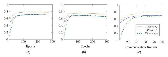
Fig. 4. Performance comparison of the centralized approach with 100% of the training set (a), centralized approach with 75% of the training set (b), and federated approach with 3 clients each using 33% of the training set (c).
