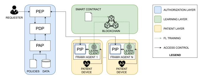
Fig. 3. The FRAMH architecture with the Authorization, Patient, and Learning layers highlighted with different colors.
