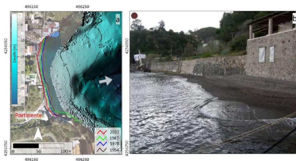
Figure 12. Map of Baia Portinente beach and related reconstructed shorelines (a) and image of the setting in November 2017 (b); see Figure 1 for location. White arrow shows the active canyon heads located in the nearshore.
