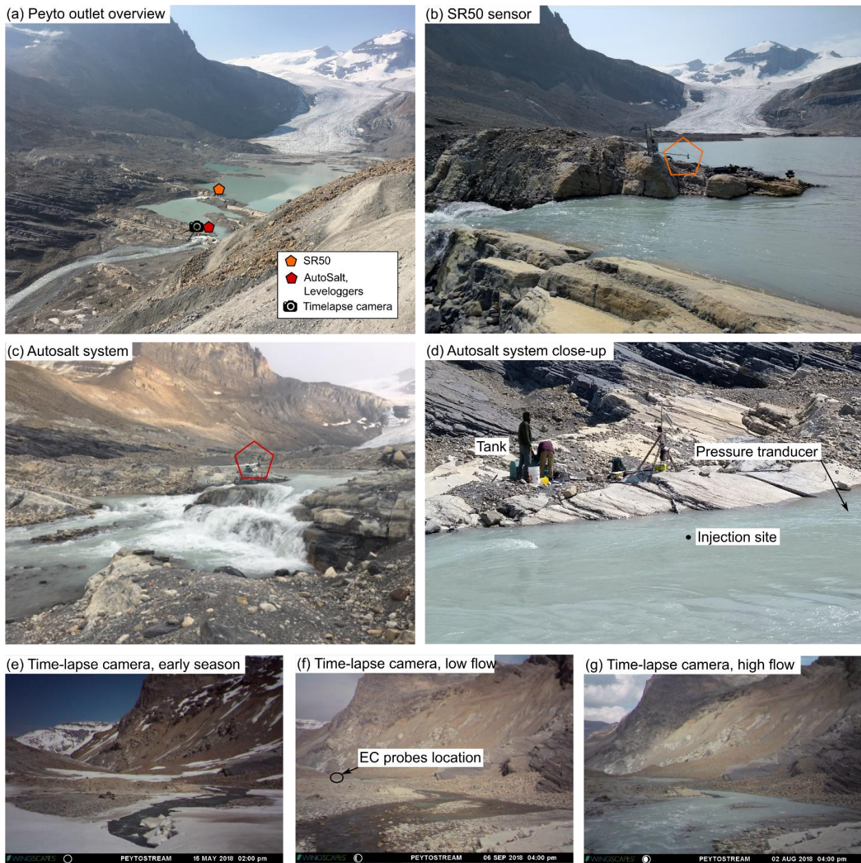
Figure 2.1. Peyto Glacier Outlet Creek area and instrumentation: (a) overview of the Peyto Glacier Research basin area, (b) SR50 sensor, (c) location of the AutoSalt system, (d) close-up view of the AutoSalt injection site and pressure transducer location and (e-f) time-lapse camera images showing early season conditions with snow blocking the channel, low flow conditions on September 6, 2018, at 4:00 PM and high flow condition on Aug. 2 nd , 2018 at 4:00 PM. The time-lapse images show the mixing reach length.
