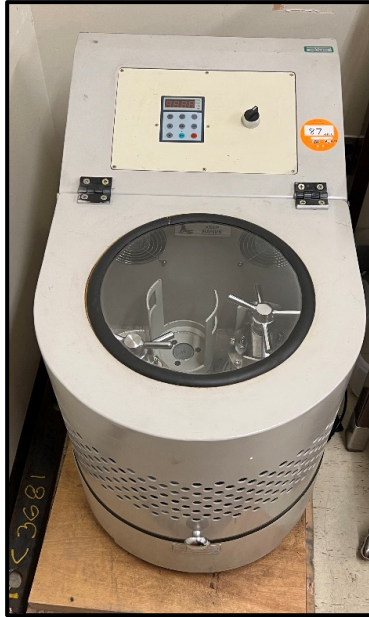
Figure 2.3: The planetary ball mill apparatus (Torrey Hills Technologies, USA) located at Department of Mechanical Engineering, University of Saskatchewan.
