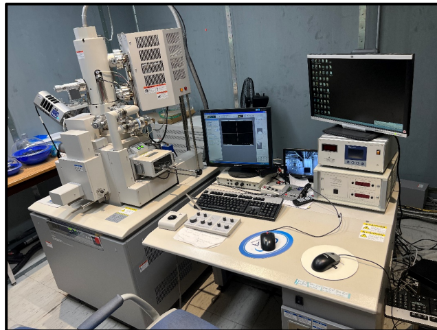
Figure 2.9: The SU-6600, Hitachi field emission SEM equipped with the Oxford Instruments Nordlys EDX detector located at Department of Mechanical Engineering, University of Saskatchewan.
