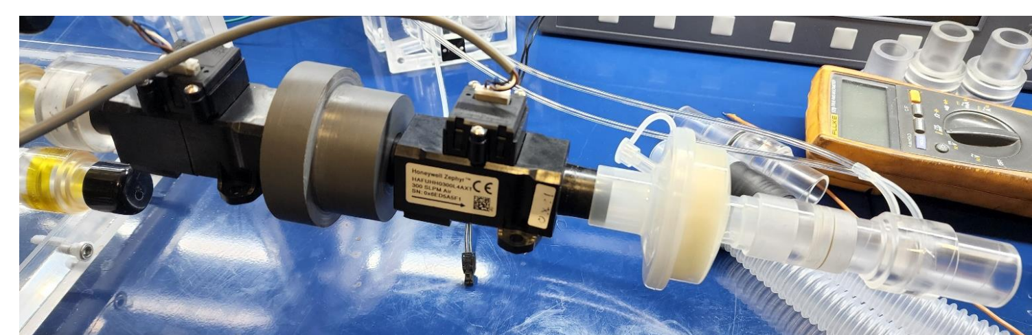
Figure 1. Experimental setup: two Zephyr flow meters (black) and RMD flow meter (clear) in series
