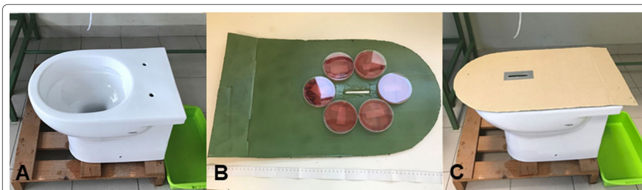
Fig. 1 Experimental equipment used to reproduce bacterial contamination: a toilet with 2000 mL of bacteria-containing solution poured into it, a tube (internal diameter: 4 mm) through which to pour 500 mL of sterile saline solution (A), a toilet cover fitted six MacConkey agar plates (B) affixed to the side facing the inside of the toilet bowl (C)
