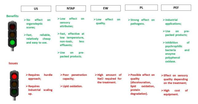
**Figure 1.** Benefits and issues of non-thermal approaches to prolong the shelf-life of fish. US, ultrasound; NTAP, non-thermal atmospheric plasma; EW, electrolyzed water; PL, pulsed light; PEF, pulsed electric field.
