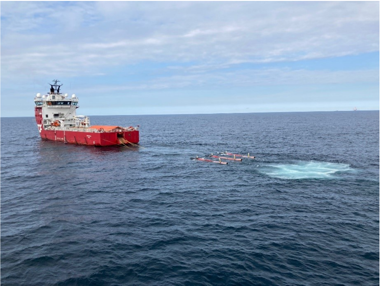
Figure 14. Showing the seismic vessel, Skandia Nova, and its airgun. Picture by Anne Christine Utne Palm.
