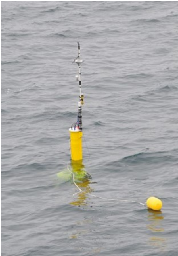
Figure 12. Hydrophones used on the cruise. Top: The Ocean Sonic Eth-X2 hydrophone, used for measuring sound during the Seismic shooting approach at the three WBAT stations. Middle and bottom: The hydrophone buoy, that contained two omnidirectional hydrophones (Naxys 02345, frequency range: 5 Hz to 300 kHz, sensitivity: -179 dB re V/ \mu Pa). The hydrophone buoy was sat out for 24h during which there were hours with and without seismic shooting. Picture top from web page, middle by Karen de Jong and bottom by Anne Christine Utne Palm.
