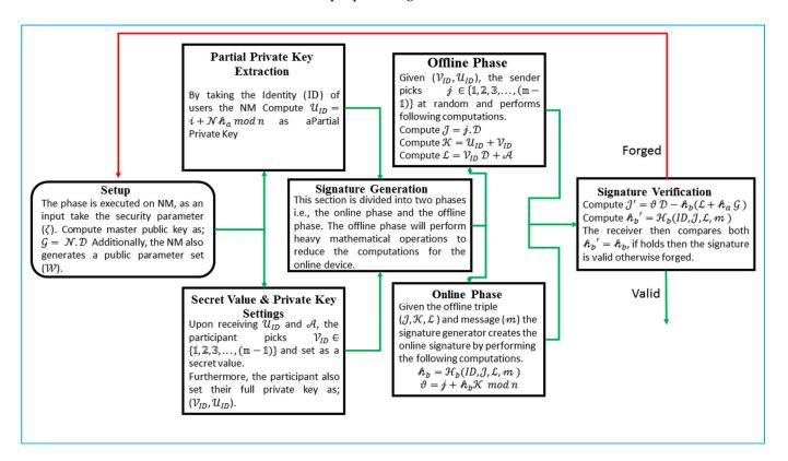
Figure 3. Flowchart of the proposed algorithm.
