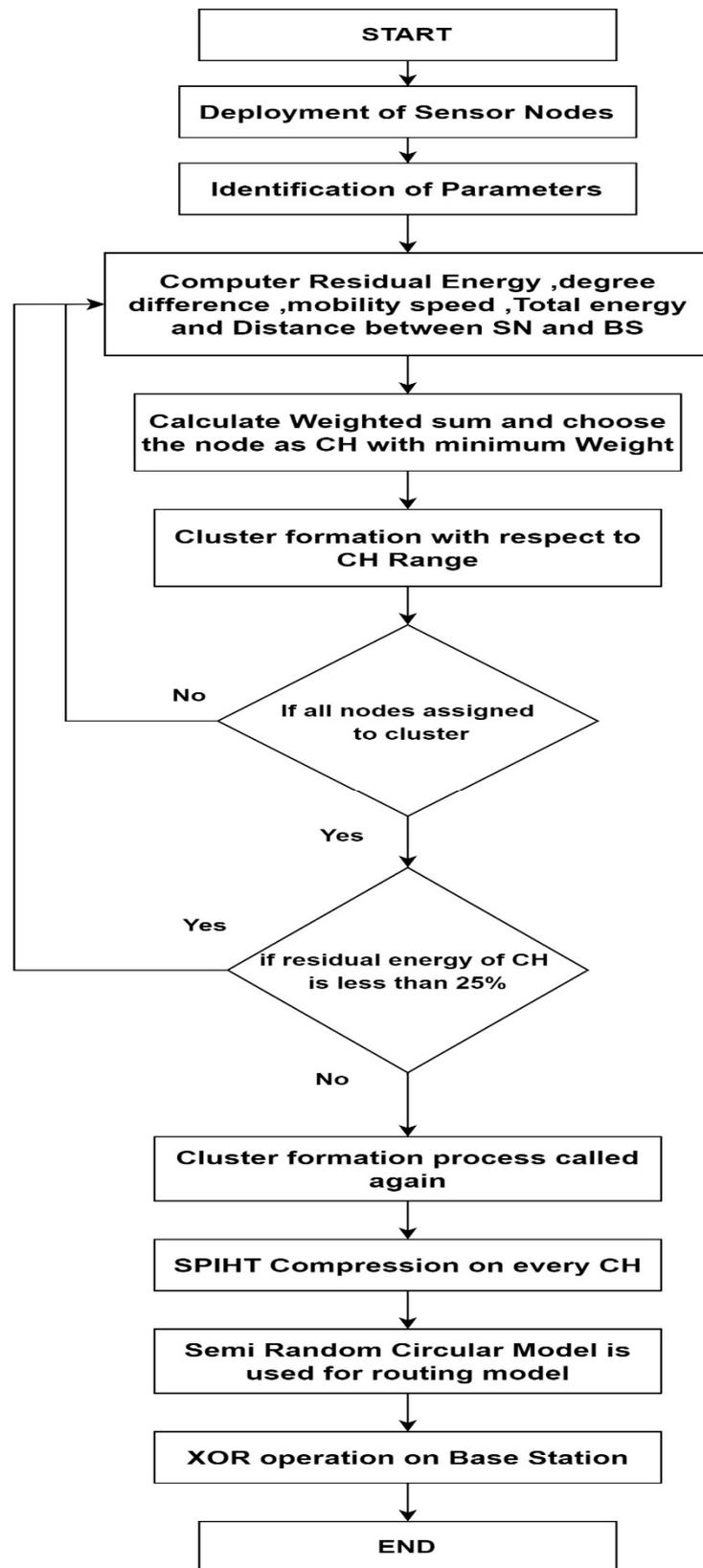
Figure 3. EE-SS proposed algorithm flowchart.
