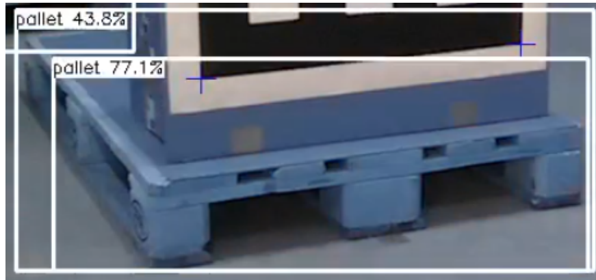
Figure 6.7: Faulty object detection during RGB to BGR bug.
