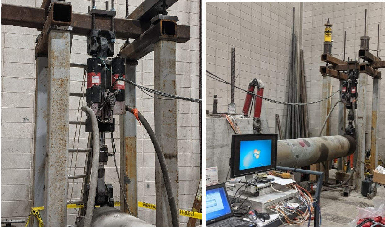
Figure 3.5. Hydraulic actuator (left) and data acquisition system and loading frame (right)
