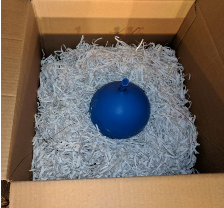
Figure A-4 Balloon Filled with 500mL of Ethanol Placed on Top of Shredded Paper
