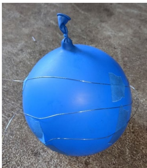
Figure A-3 500mL of Ethanol in a Balloon with Nichrome Wire Wrapped Around
