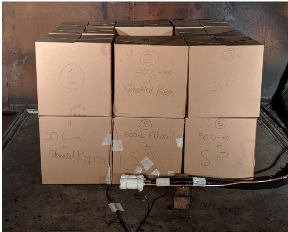
Figure A-7 Challenge Fire Test Setup without Rain Wrap
