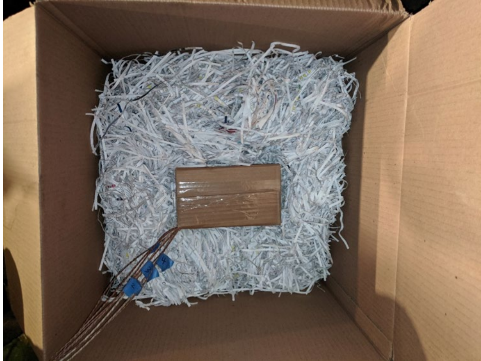
Figure A-6 Lithium-ion Cells Package Placed on Top of Shredded Paper
