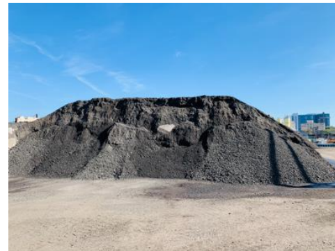
(b) Recycled Asphalt Pile
