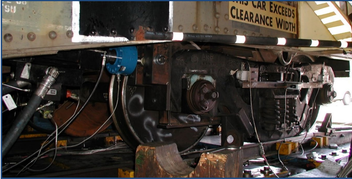
Figure 4. “Standard Warp Test” setup and configuration Note: The blue load cell of a longitudinal actuator is seen between the side frame and carbody.
