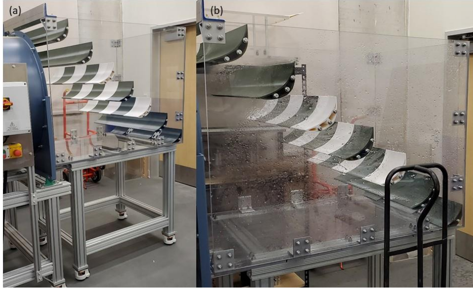
Figure 22. Flow turning vanes and droplet capture system: (a) System as installed and (b) System in operation during a cloud LWC uniformity test
