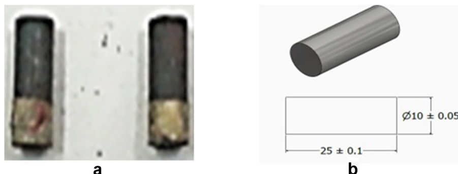
Figure 1. (a) Actual specimen for chemical composition and (b) Specimen diagram with measurement for chemical composition.
