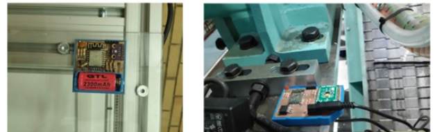
Figure 2. Sensing modules installed in the metal stamping machine.
