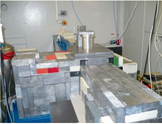
Fig. 1. The PGAA facility at Garching. Lower right corner: shielding of the beam stop, left side: shielding and dewar of the detector, in the middle: sample chamber tube.
