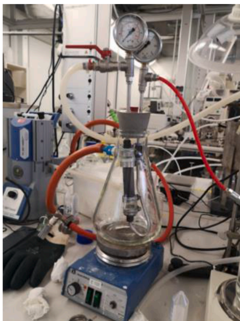
Fig. A1. A picture of the percrystallization set up used in the study for testing Si-C membranes.
