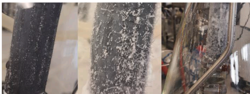
Fig. 9. (a) The surface of MP3 after a few minutes of percrystallization where initial NaCl crystals are clearly visible. (b) needle shaped NaCl crystals clearly visible after ~ 20 min of percrystallization (c) the crystals obtained after running the experiment multiple times.
