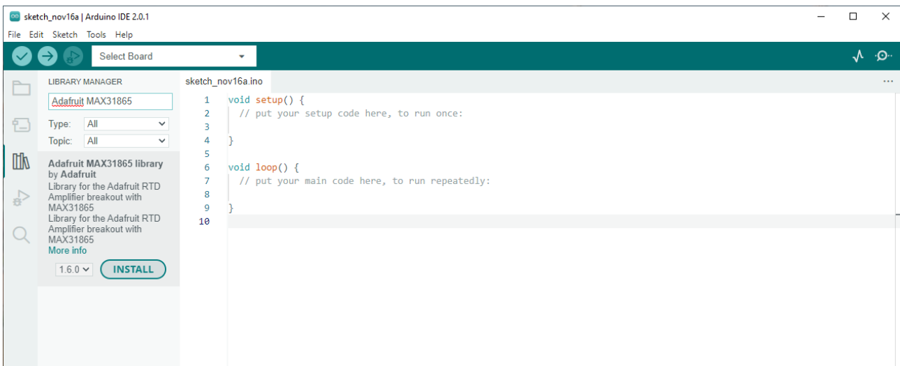
Figure 19. Library manager and the relevant library for the code used in this setup (Adafruit MAX31865 library).
