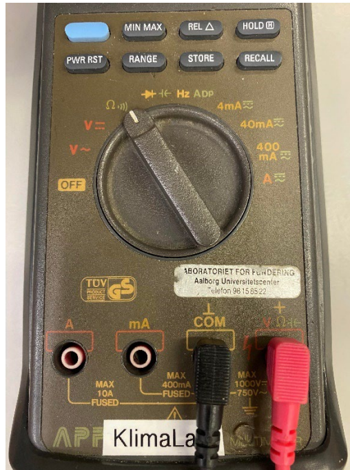
Figure 27. Multimeter with the knob placed to measure resistance and continuity.
