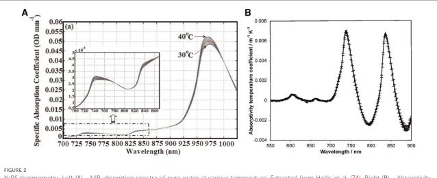
NIRS thermometry. Left (A) - NIR absorption spectra of pure water at various temperature. Extracted from Hollis et al. (74). Right (B) - Absorptivity temperature coefficients (da/dT) for the 550–900 nm. Extracted from Langford et al. (75).
