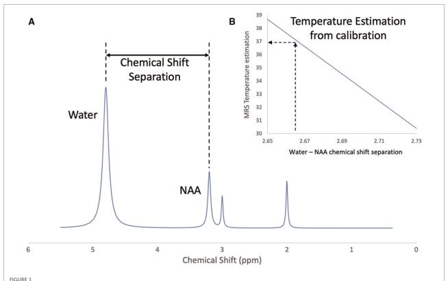
Brain temperature measurement using proton magnetic resonance spectroscopy. (A) Indicates the chemical shift separation between the water peak and a reference metabolite (NAA), (B) represents the calculation of brain temperature using a calibration based on the water-NAA chemical shift separation.
