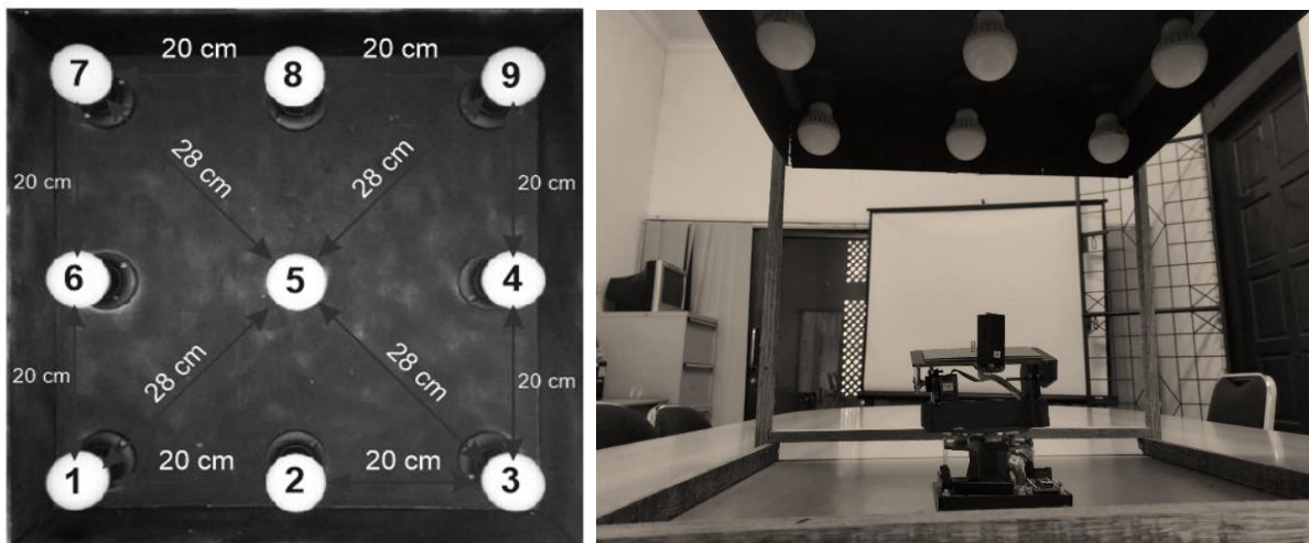
Gambar 5. (a) Jarak antar lampu (b) Simulator matahari
