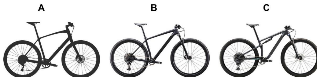
Figure 8 - Rigid (A), hardtail (B) and full suspension (C) bike models for the XC-MTB events
