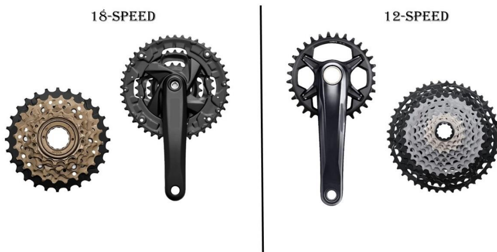
Figure 9 - Most popular in the 1990s (18-speed) and more recent (12-speed) gear system models. Although the left allows more speed combinations, the right one is more accurate, lighter, stronger, more efficient and easier to handle
