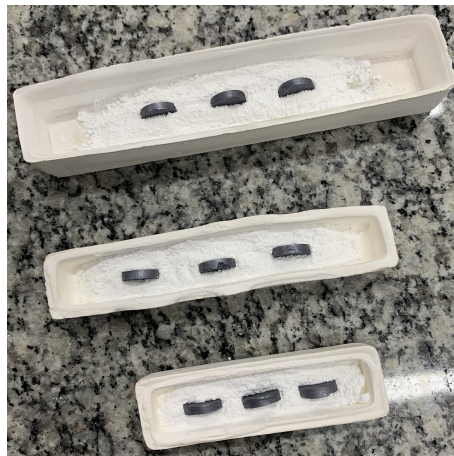
Figure 21 – Nine pellets from MoS 2 with temperatures ranging from 600 °C to 800 °C and pressures considering a load of 10 T to 20 T.
