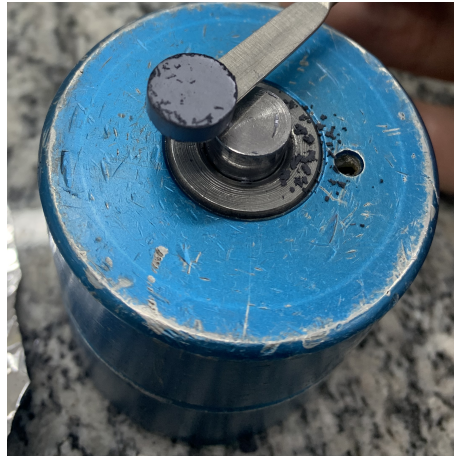
Figure 20 – Pellet after being compacted in the Pellet Press Die Set.
