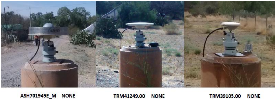
Figura 2. Antenas inclinación 0° (Ashtech Choke Ring, Trimble Zephyr Geodetic, Trimble Zephyr). Figure 2. Tilt antenna 0° (Ashtech Choke Ring, Trimble Zephyr Geodetic, Trimble Zephyr).
