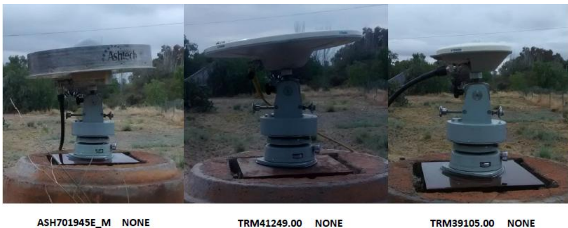
Figura 3. Antenas inclinación 5° (Ashtech Choke Ring, Trimble Zephyr Geodetic, Trimble Zephyr). Figure 3. Tilt antenna 5° (Ashtech Choke Ring, Trimble Zephyr Geodetic, Trimble Zephyr).
