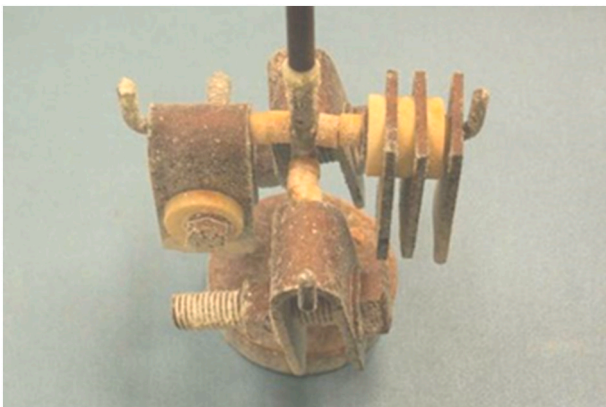
Fig. 5. Metallic tree device with uniform corrosion coupons and SCC specimens after testing.
