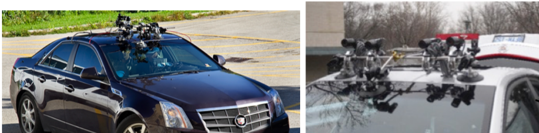
Figure 3.1: RoadLAB instrumented vehicle (left). Forward stereoscopic vision system (right).
