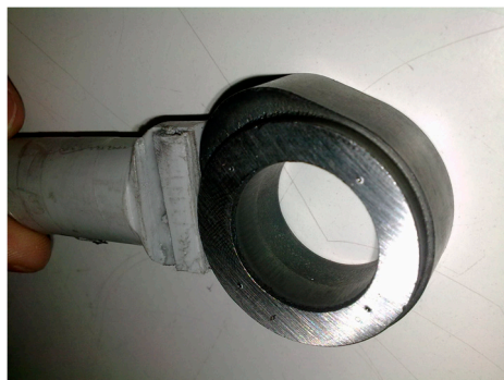
Figure 7. Image of the impedance acquisition procedure during the eddy current nondestructive tests.
