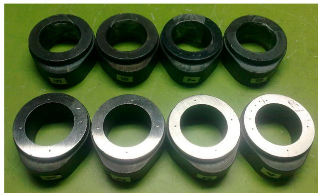
Figure 3. Image of the steel cams employed in the experiments: the four cams of the lower row (Group 1) had a predominant microstructure of martensite and a hardness greater than 55 HRC, while the four cams of the upper row (Group 2) had a predominant microstructure of perlite and a hardness lower than 45 HRC.
