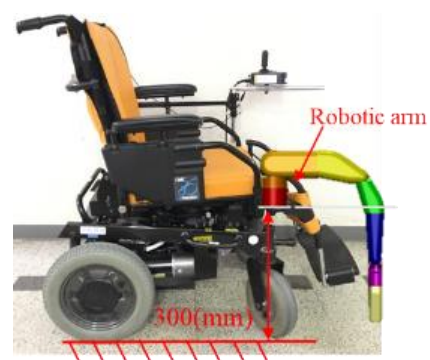
Fig. 2. Mounting position of robotic arm on wheelchair
