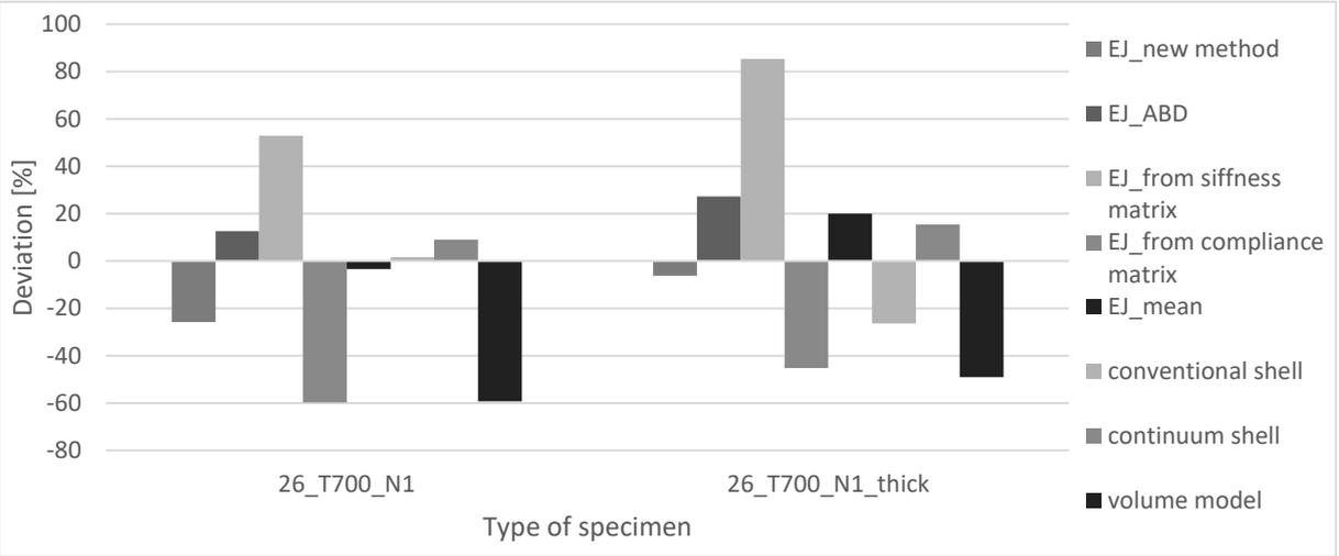
Fig. 1. The deviation from the experiment of equivalent stiffness for beams with ID 26 mm and Diagonal 1  $[90^\circ, \pm 45^\circ]$
