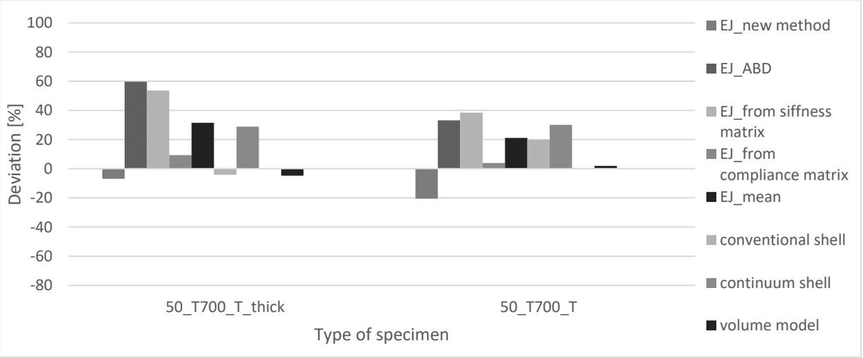
Fig. 2. The deviation from the experiment of equivalent stiffness for beams with ID 50mm and Typical layup  $[90^\circ, 0^\circ, \pm 30^\circ]$
