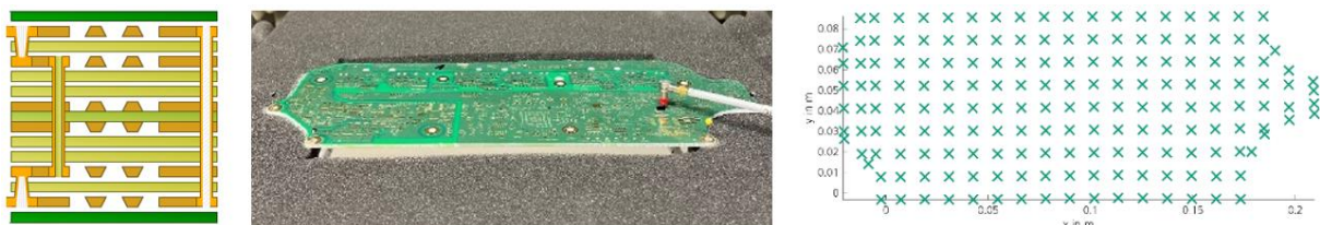
Fig. 1. PCB cross section (solder mask, copper foil, FR4 prepreg, FR4 core), measurement set-up and measurement points [4]
